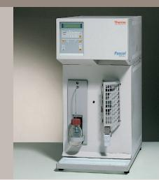
Operations are done automatically thus freeing the operator for other tasks. Thanks to its modular concept, it can be used by itself or together with other Pascal porosimeters, thus modularity of the Pascal system features a "buy what you need" approach. Data from the low pressure intrusion can be combined with data from the other high pressure modules (240 or 440) to get a complete porosity spectrum of the sample.
