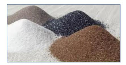
Predictably, the more aggressive the grit, the more efficiently the material is removed. However, the powder's grit is not only determined by the size of the particles, but also its shape properties. A low grit, corresponding to a more robust removal, has larger particles. Nevertheless, if these larger particles were all smooth and round, the removal effectiveness would be weak. Consequently, both size and smoothness are key factors in the performance of abrasive powders.
