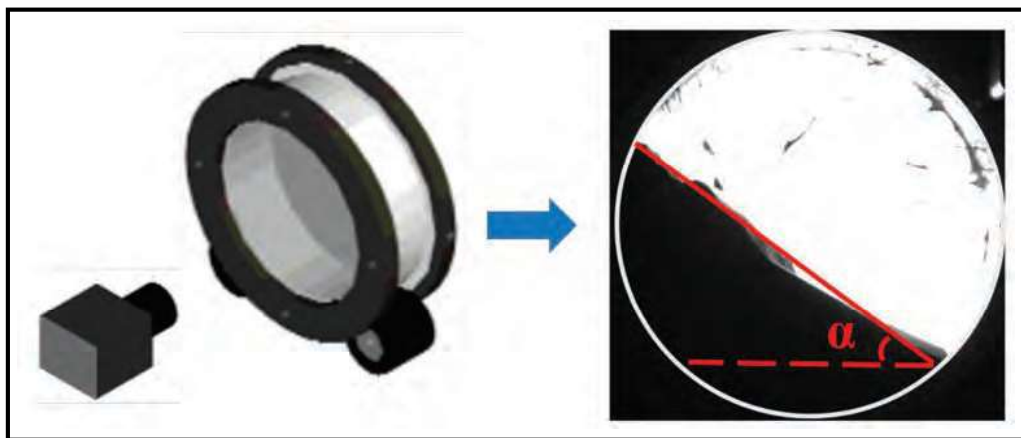
Figure 4. Illustration of working principle of rotating drum analyzer. Avalanche profile of powders is captured by a camera as the drum is rotating. The avalanche angle \alpha is measured by image analysis.
