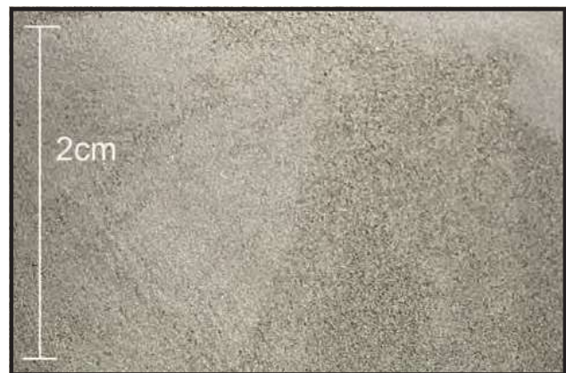
Figure 8. Image of the segregation pan top surface for Sample B Recycled after sifting. Larger particles can be seen on the top surface
