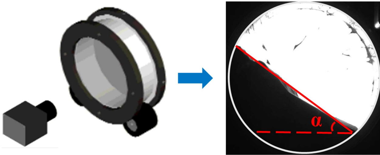
Figure 4. Illustration of working principle of Revolution Powder Analyzer. Avalanche profile of powders is captured by a camera as the drum is rotating. The avalanche angle \alpha is measured by image analysis
